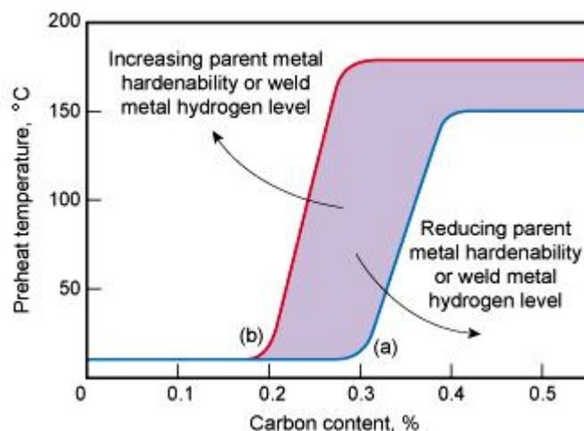
Fig.1 Guide to preheat temperature when using austenitic MMA electrodes at 1-2kJ/mm a) low restraint (e.g. material thickness <30mm) b) high restraint (e.g. material thickness >30mm)
