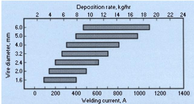
SAW is usually operated as a fully-mechanised or automatic process, but it can be semi-automatic. Welding parameters: current, arc voltage and travel speed all affect bead shape, depth of penetration and chemical composition of the deposited weld metal. Because the operator cannot see the weld pool, greater reliance must be placed on parameter settings.
