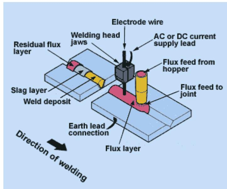
The first patent on the submerged-arc welding (SAW) process was taken out in 1935 and covered an electric arc beneath a bed of granulated flux. Developed by the E O Paton Electric Welding Institute, Russia, during the Second World War, SAW's most famous application was on the T34 tank.
